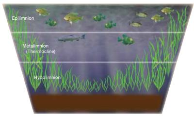
**STRATIFIED WITHOUT AERATION** — Warm, typically oxygen rich water floats on top of a cooler and less oxygenated middle layer. The bottom of the pond is typically dense with weeds, cold and completely void of dissolved oxygen.
